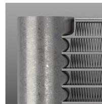
**5 OVER-CORE REINFORCEMENTS**— For added protection, over-core reinforcements on the top and bottom of the coil are twice as thick as internal tubes and do not circulate refrigerant.
