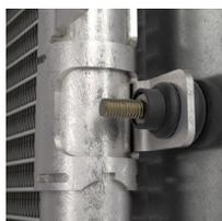
**2 COIL MOUNTING ISOLATORS**—Rubber inserts help to reduce vibration. Plus, the isolators prevent corrosion by separating the coil from the rest of the unit and eliminating metal-to-metal contact.
