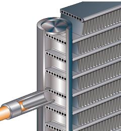
a flat extrusion tube, fins in-between the flat extrusion tubes and two refrigerant manifolds.
