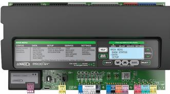
The Intelli-Guide™ unit controller is a microprocessor-based controller that provides flexible control of all unit functions.
