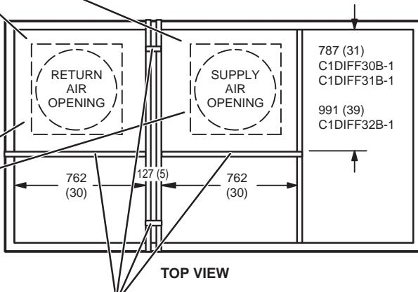
NOTE - These four supports are furnished with the transitions to replace supports furnished with curb for proper transition spacing.
