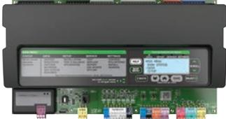
The Intelli-Guide™ unit controller is a microprocessor-based controller that provides flexible control of all unit functions.
