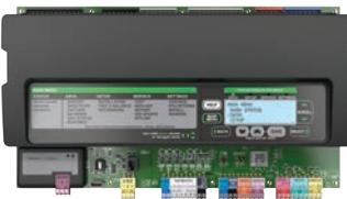
The Intelli-Guide™ unit controller is a microprocessor-based controller that provides flexible control of all unit functions.
