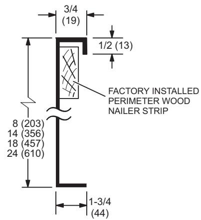
ADJUSTABLE PITCH ROOF CURB
