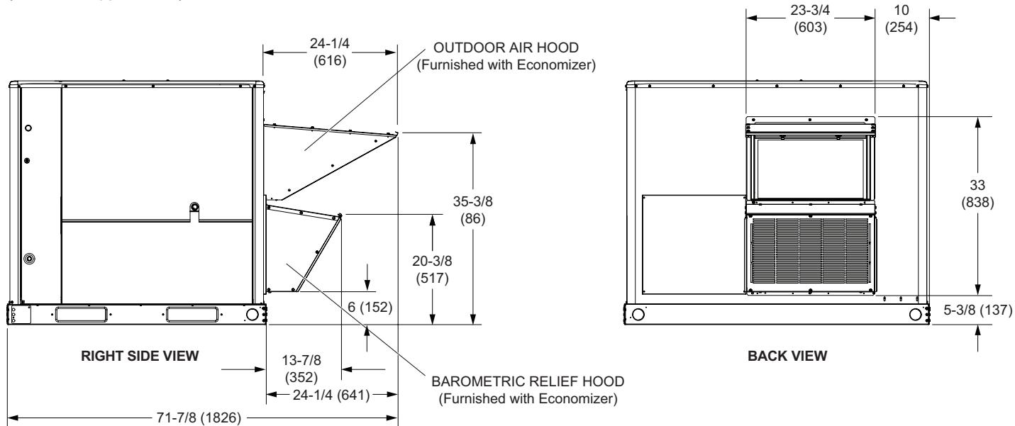
**OUTDOOR AIR HOOD DETAIL FOR OPTIONAL ECONOMIZER WITH BAROMETRIC RELIEF DAMPERS**
