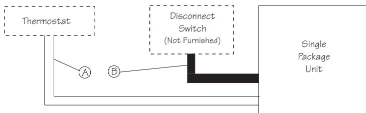
A - \*Four Wire Low Voltage (Electro-mechanical)
