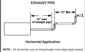
**NOTE:** All horizontal runs of exhaust pipe must slope back toward unit. A minimum of 1/4" (6 mm) drop for each 12" (305 mm) of horizontal run is mandatory for drainage.
