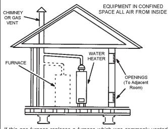
If this gas furnace replaces a furnace which was commonly vented with another gas appliance, the size of the existing vent pipe for that gas appliance must be checked. Without the heat of the original furnace flue products, the existing vent pipe is probably oversized for the single water heater or other appliance. The vent should be checked for proper draw with the remaining appliance.
