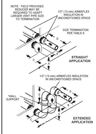
See venting Table 5 for maximum venting lengths with this arrangement.
