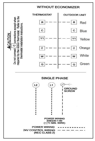
Figure 6. Typical Wiring Connections
