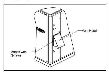
Figure 2. Installing the Vent Cover
