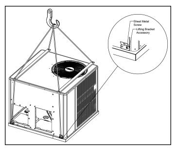
Figure 1. Rigging Unit
