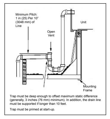
**Figure 3. Typical Condensate Drain Connection**
