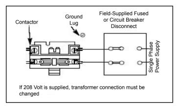
Figure 5. 208/230 Line Voltage Wiring
