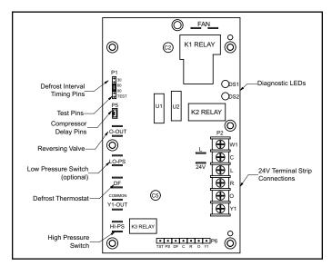
Figure 8. Defrost Control Board
