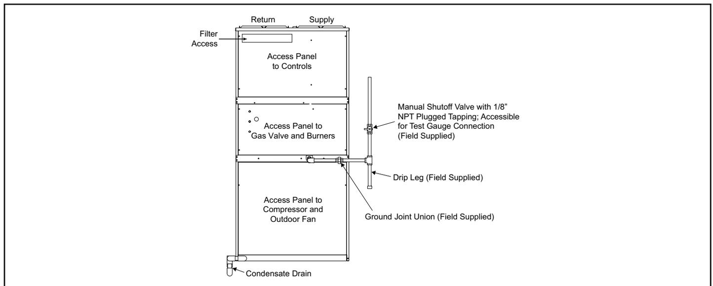
**Figure 7. Gas Supply Piping**
