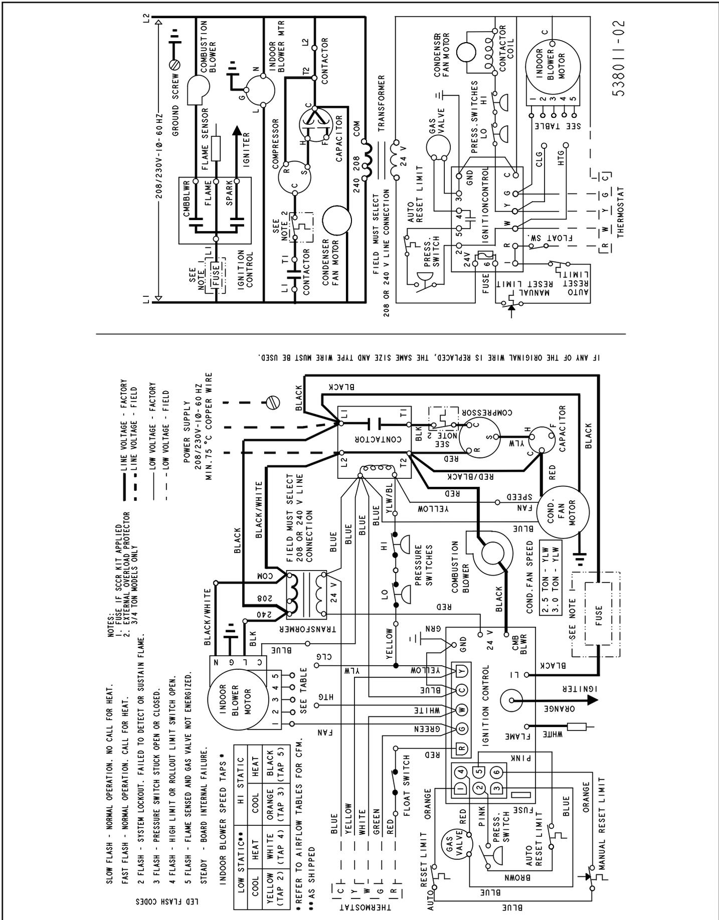
Figure 10. Wiring Diagram - 2-1/2 Ton and 3 Ton
