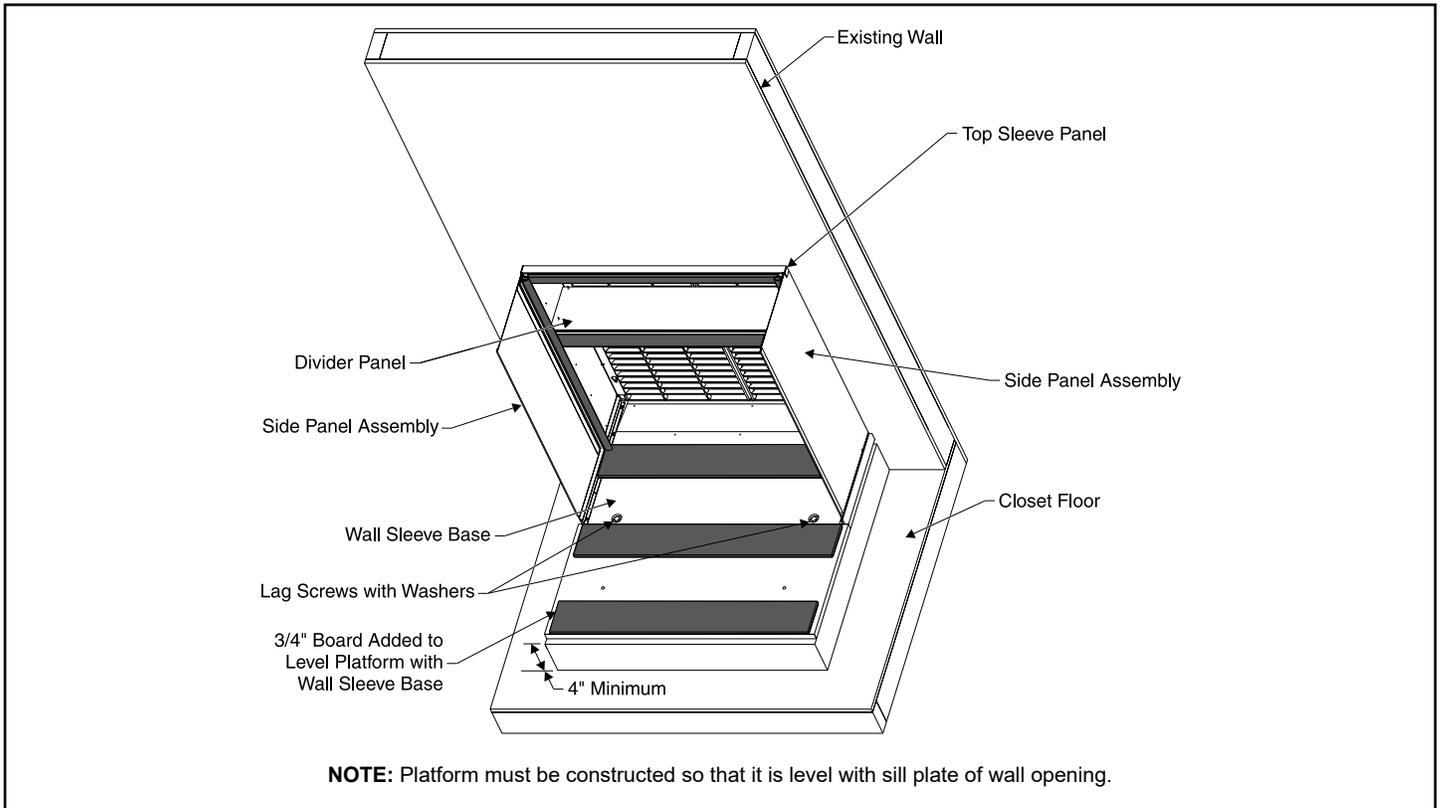
**Figure 2. Wall Sleeve and Louver Kit Installed**
