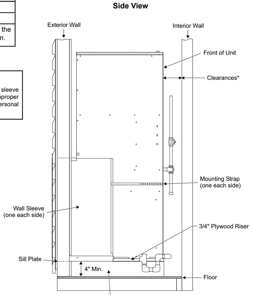
**Platform (field supplied) must be level with sill plate of hole in exterior wall. Unit must be supported by platform.**
