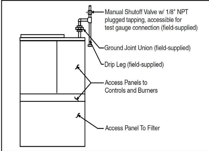
**Figure 3. Gas Supply Piping**
