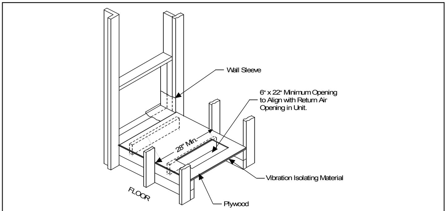
**Figure 1. HWC Installation**
